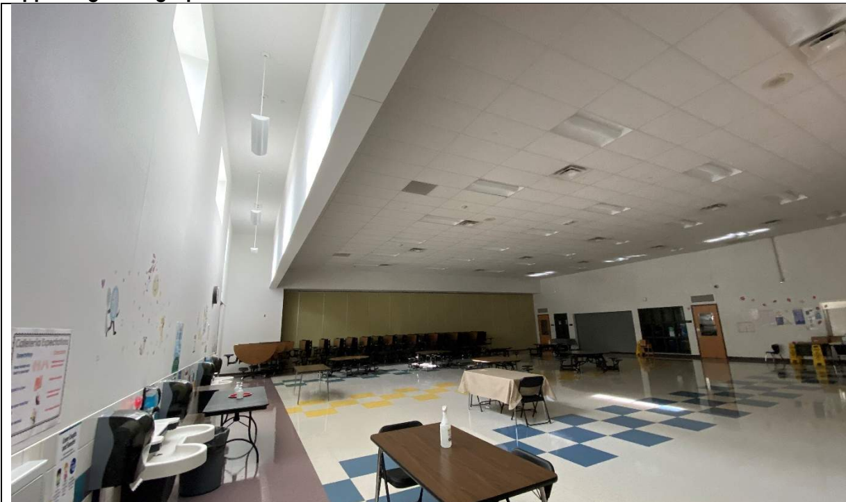
Food Services: Clerestory windows let natural light into the cafeteria. An operable partition connects to the gym in the back.
