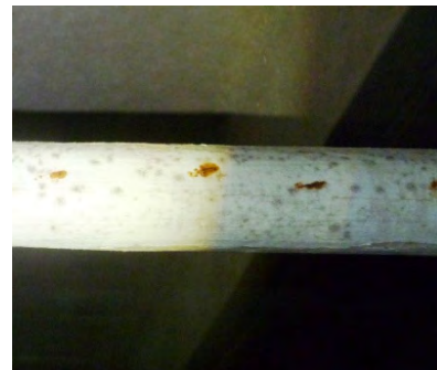
Rusting pipes behind insulation
