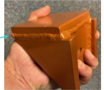
Strike plate mounted on the side of the beam near the test pile
