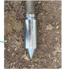
Sensors before placing in the borehole
